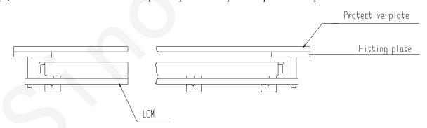
(2) When assembling the LCM into other equipment, the spacer to the bit between the LCM and the fitting plate should have enough height to avoid causing stress to the module surface, refer to the individual specifications for measurements. The measurement tolerance should be  $\pm 0.1$ mm.
