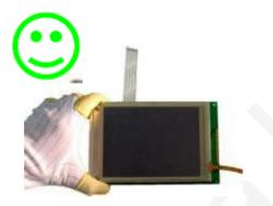
As above picture, please handle with anti-static gloves around LCM edges.
